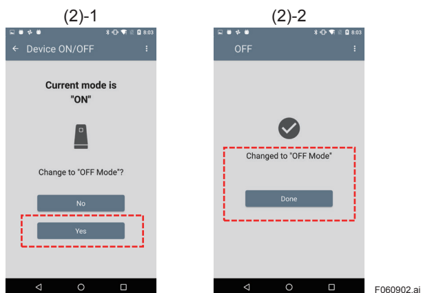
Figure 6-13 Shifting XS770A to OFF Mode
