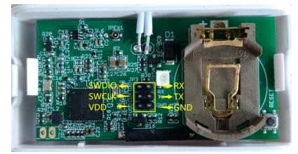
USB to TTL <- -> LWL01 RX <- -> TX TX <- -> RX GND <- -> GND
